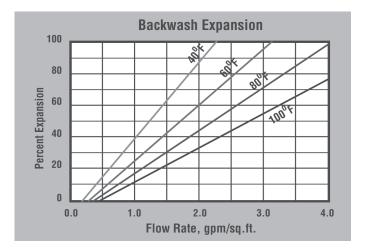
**BACKWASH** — After each cycle the resin bed should be backwashed at a rate that expands the bed 50 to 75 percent. This will remove any foreign matter and reclassify the bed. The graph above shows the expansion characteristics of ProSelect Silica in the chloride form.
